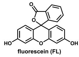
redox potentinal (vs Ag/AgCl) [FL]\*/[FL]<sup>--</sup> = + 0.81 V, [FL]<sup>+/</sup>[FL]\* = - 1.03 V [*p*-MeOCH<sub>2</sub>PhB(OH)<sub>3</sub>]<sup>-</sup>[*p*-MeOCH<sub>2</sub>PhB(OH)<sub>3</sub>]<sup>-</sup> = + 0.85 V O<sub>2</sub>/[O<sub>2</sub>]<sup>--</sup> = - 0.83 V
