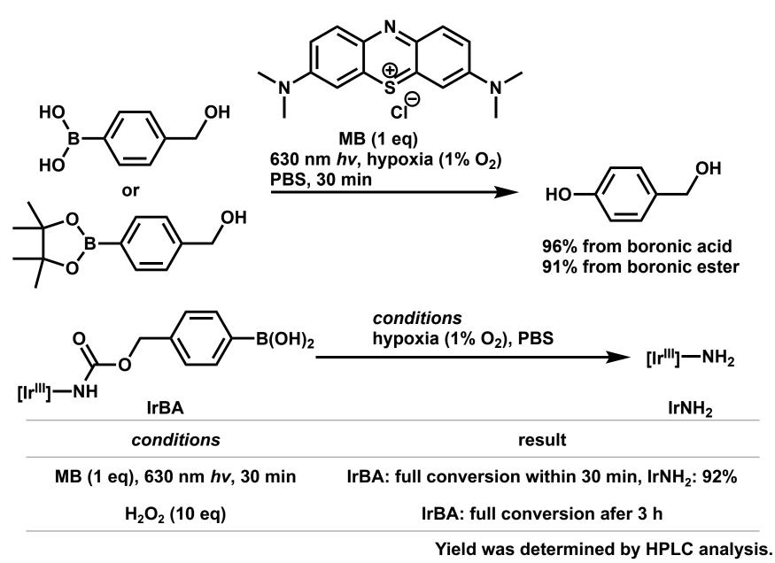
Boronic acids and esters were successfully uncaged by MB and 630 nm hv under hypoxia.
