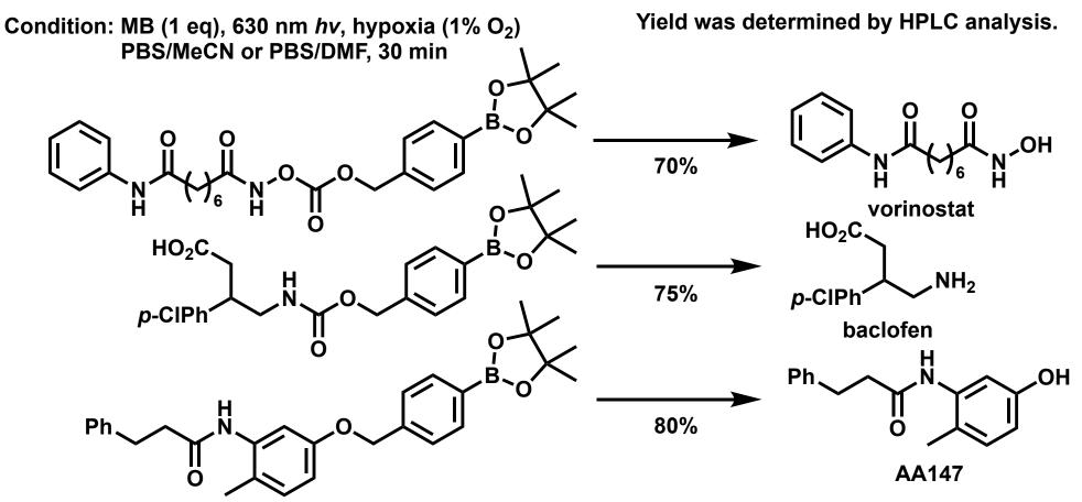
Three prodrugs were uncaged by MB and 630 nm hv under hypoxia.
