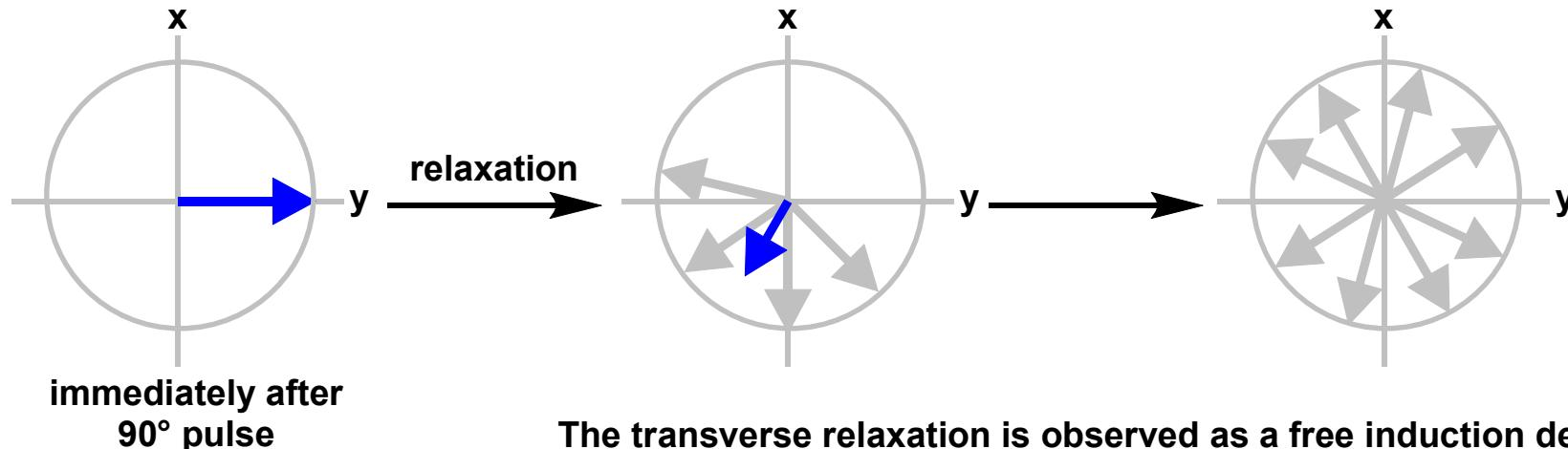
The transverse relaxation is observed as a free induction decay (FID). NMR machine measures this FID.
