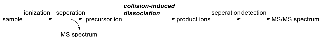
Figure 2. MS/MS analysis using collision-induced dissociation. Multiple tandem mass spectrometry (e.g. MS 3 , problem 1) is possible by further degradation/separation/detection of product ions.
