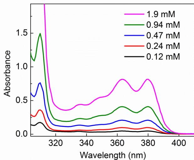
**Fig 5. UV-vis spectra of  $[\text{Cu}(\text{carb})_2]\text{Li}$  absorption at 365 nm with  $\epsilon = 4300 \text{ M}^{-1} \text{ cm}^{-1}$**
