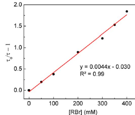
**Fig 6. Stern-Volmer plot of  $[\text{Cu}(\text{carb})_2]\text{Li}^*$**
