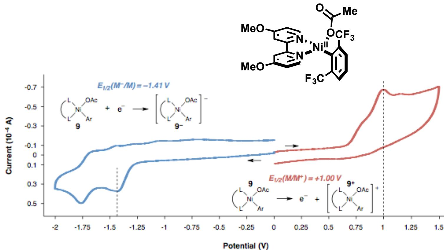
**Figure S11.** Cyclic voltammetry suggests against a redox-induced mechanism.
