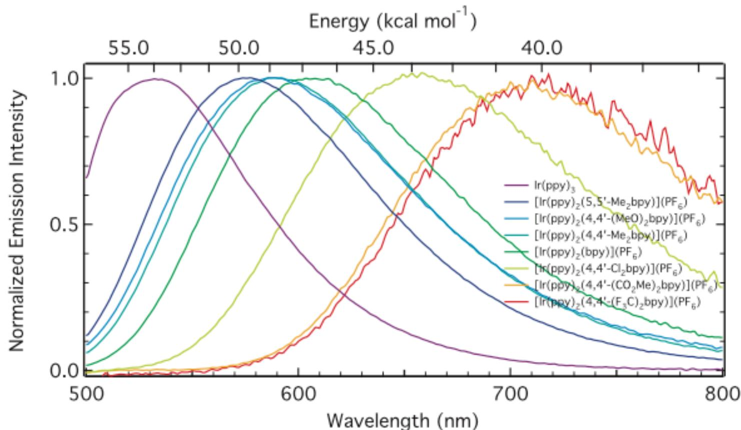
**Figure S9.** Emission spectra were converted from wavelength to energy units (59). E(<sup>3</sup>MLCT) were calculated by a single mode fit of the steady-state emission spectrum, as described by Claude and Meyer (60). Excited state oxidation potentials ( $E_{1/2}^{\text{II/III}^*}$ ) were calculated as described in reference 14.
