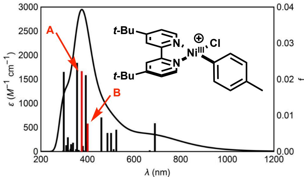
Fig. 1. Calculated absorption spectrum (solid black line) and oscillators (solid bars; red bars: transitions with  $> 10\%$  Ni–Cl,  $\sigma \rightarrow \sigma^*$  contributions) from TD-DFT calculations on  $[\text{Ni}^{\text{III}}(\text{dtbbpy})(\text{Ph})\text{Cl}]^+$ .
